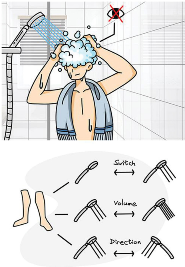
Figure 1. An illustrative scenario of eyes-free interaction in a smart shower room. The user is shampooing with eyes closed, and he performs foot gestures to achieve eyes-free interaction with smart shower devices naturally and conveniently.
